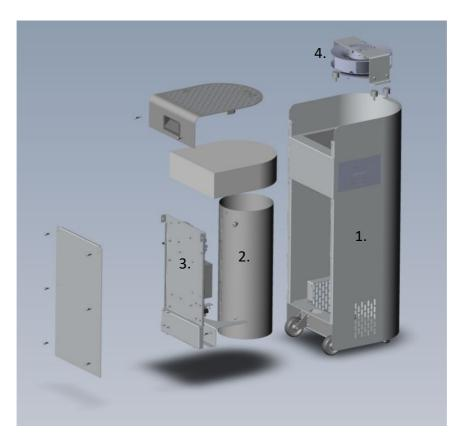
**Figure 6.** Genano 360 main components for recycling: 1. Chassis materials, electronics base plate and collector tube, 2. Collector tube, 3. Electronic components and cables, 4. Fan unit.
