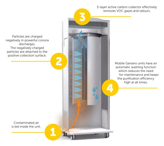
Outcoming ultrapure air is completely free from particles of all sizes, microbes, and harmful gases and chemicals.
